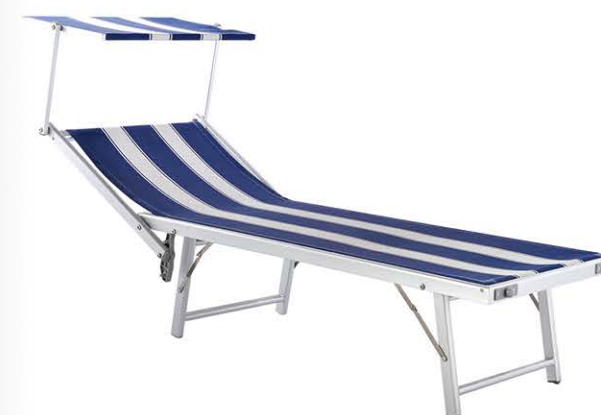
AB1001 AI ++ ☑ Feature: Sun Lounge. Adjustable back rest with sun shade. 2-positions. ■ Fabric: 650g Textilene ▲ Frame: 43x42mm, 42x25mm Alu. tube/matt finish 📏 Dimension: 186X61X38cm 📦 Packing: 153X10.5X72.5cm/1pcs
