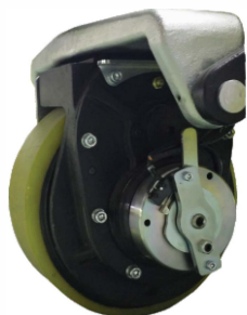
Optional Releasable Brake To use it exactly like hand pallet truck for special applications
